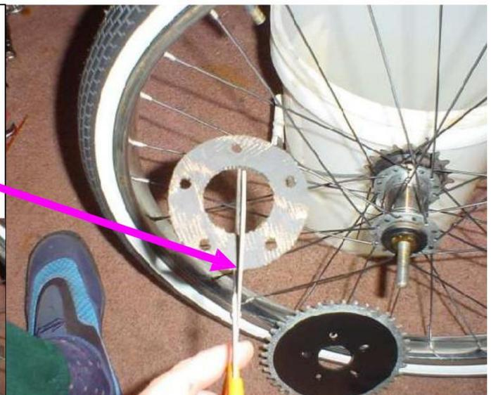
**Note:** A joint binder may be needed on both sides of the sprocket for chain alignment on some non-coaster brake bikes.
