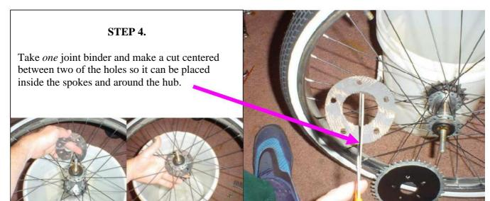
**Note:** A joint binder may be needed on both sides of the sprocket for chain alignment on some non-coaster brake bikes.
